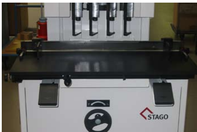
PB 5010 fitted with two-hand control
